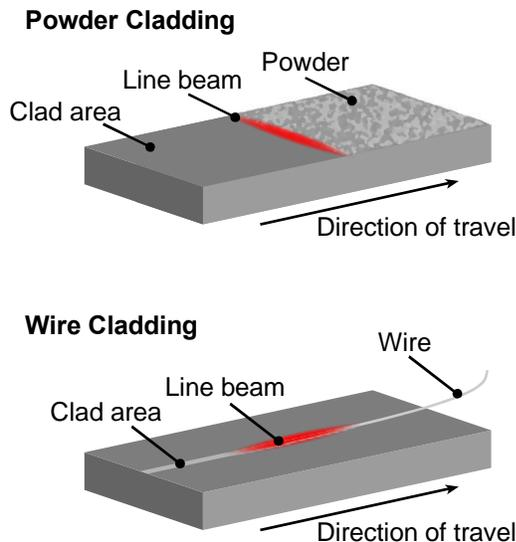
**Figure 7.** Typical configurations for powder and wire cladding using the line beam output from a high power diode laser system.
