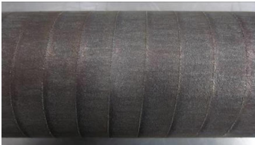
**Large Area Cladding of Stainless Steel Shaft**
