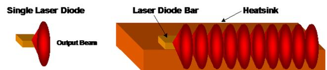
**Figure 2** Diode laser bars consist of multiple individual emitters on a single, monolithic substrate, each producing a divergent cone of light.
