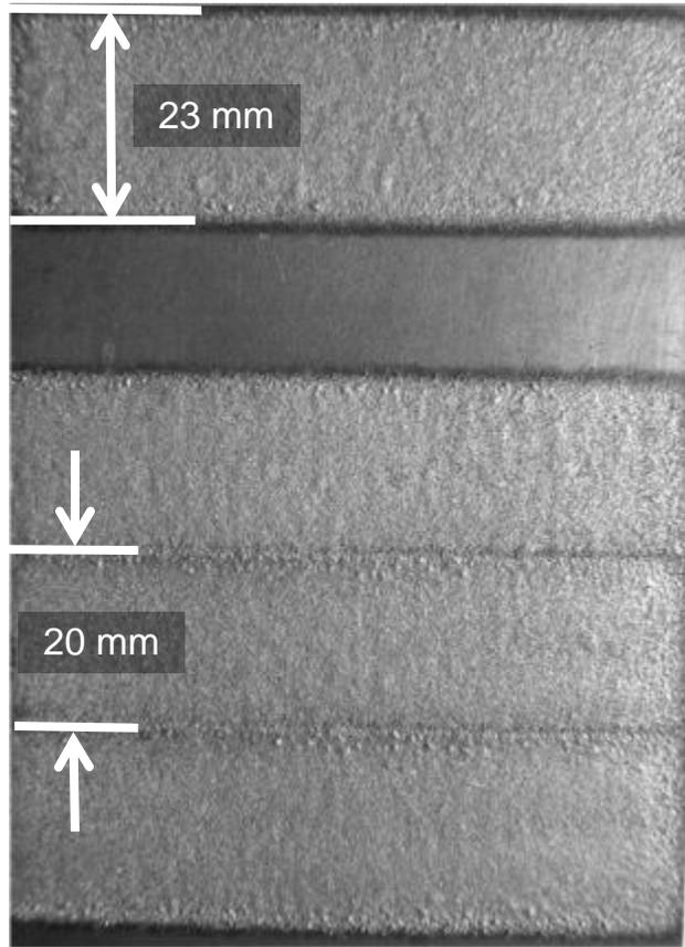
**Thin Layer Ni-WC Clad (60%) Deposit**
