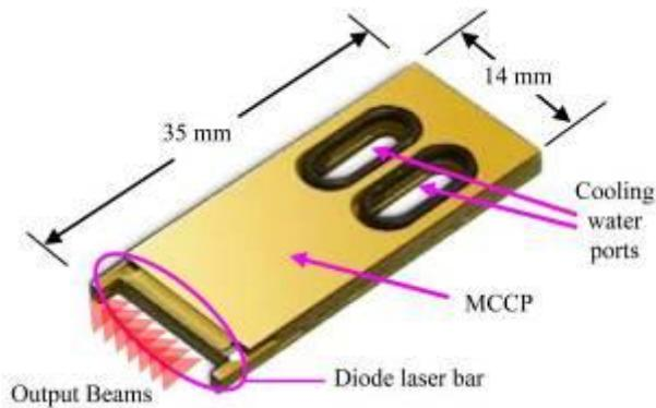
**Figure 3.** A single diode laser bar mounted on a MCCP.
