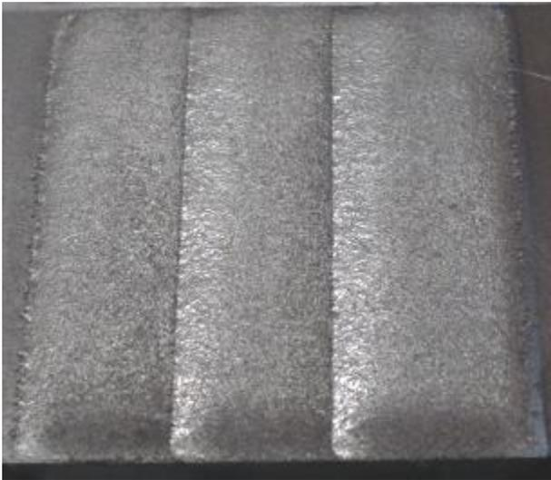
**Large Area Cladding of Steel Plate with new HighLight D-Series Laser System**
