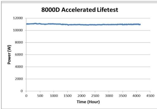
**Figure 6.** Coherent HighLight 8000D (8 kW) laser life test data which extrapolates to an anticipated diode array lifetime (MTTF) exceeding 20,000 hours
