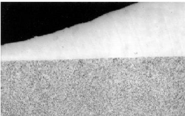
**Figure 1.** Photo of the clad cross section shows essentially no dilution of the substrate material.
