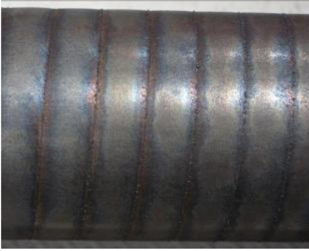
**Large Area Cladding of Stainless Steel Shaft**
